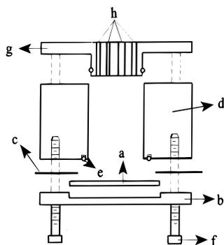
**Figure 1.** Schematic cross-sectional representation of the electrochemical cell utilized in this investigation: (a) ITO electrode, (b) base assembly, (c) aluminum foil electrical contact, (d) plexiglass cell body (e) O-ring, (f) four screws for cell assembly, (g) cell cap, and (h) ports for reference and auxiliary electrodes and for nitrogen inlet and outlet.
